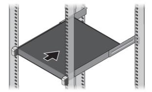
Install the system into a rack.
