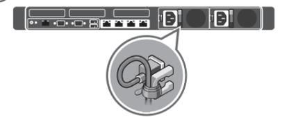
Loop and secure the power cable using the retention clip.
